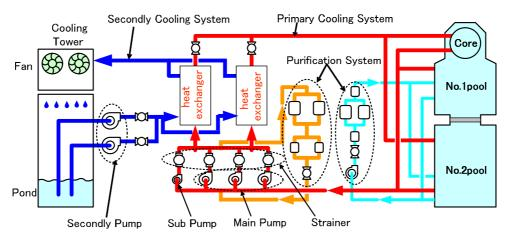
Fig 4. Cooling system of JRR-4
