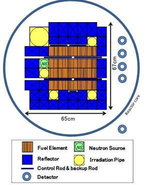
Fig 3. Layout of the reactor core of JRR-4
