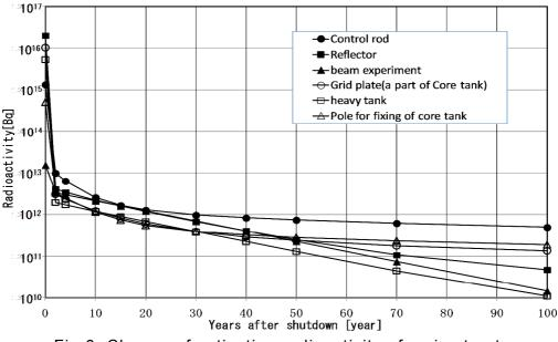
Fig.6. Change of activation radioactivity of main structures
