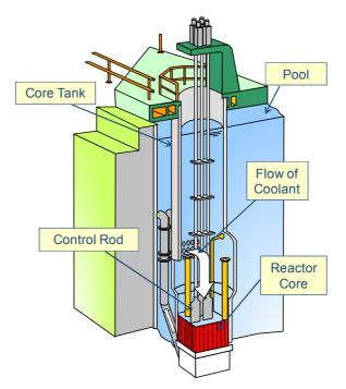
Fig 2. Cutaway view of the core tank of JRR-4
